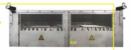
Underfloor resistor with convection cooling for installation under a subway / underground train in 3PQ4 design
